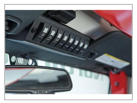
The first three switches on the sPOD can now be labeled to coincide with our wires in the sPOD module.
