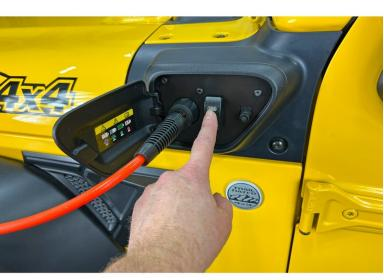
Toggle the compressor switch to the on position. The compressor should turn on for a short period
