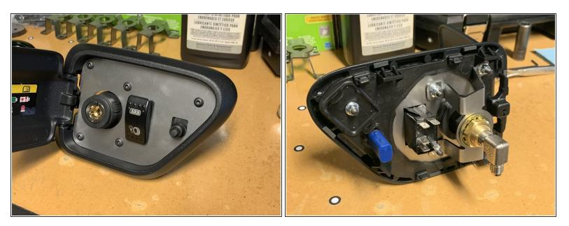
Push the ARB switch into the bracket until you hear it snap into place.
