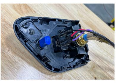
Plug the wires from the Grimm OffRoad supplied switch wire harness into the back of the ARB compressor switch. The BLACK wire goes to the top terminal, the RED wire goes to the center terminal and the PURPLE wire goes to the lower terminal.
