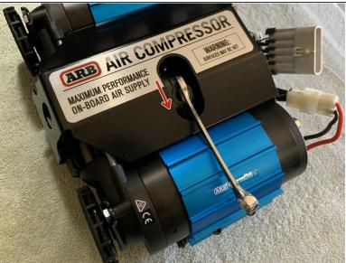
To optimize air line route, loosen manifold cap with 10mm box end wrench and rotate housing 15deg. Once adjusted, tighten manifold cap to approximately 7 lb-ft (9 Nm)
