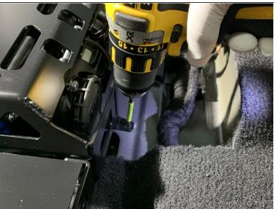
Mark a 3/16" drill bit to a depth of about 9/16" to prevent from drilling too deep.
