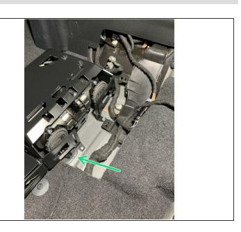
To seal the hole in the floor from the grommet removed earlier, cut a hole in the grommet for the wires to pass through and reinstall.
