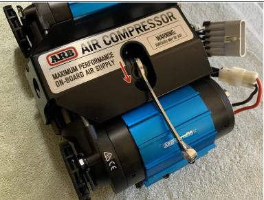
To optimize air line route, loosen manifold cap with 10mm box end wrench and rotate housing 15deg. Once adjusted, tighten manifold cap to approximately 7 lb-ft (9 Nm)
