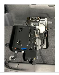
Connect the ARB Power Harness to the compressor bracket assembly and place back in the vehicle.
