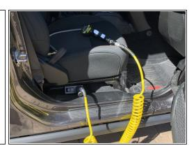
Toggle the compressor switch to the on position. The compressor should turn on for a short period of time then turn off.
