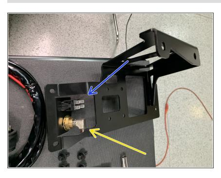
Install the 90 degree 1/4" NPT x JIC4 fitting into the back of the bulkhead fitting on the Compressor Mounting Bracket Assembly using a 9/16" open end wrench. Use thread sealant on the NPT threads.
