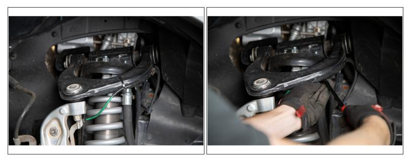
• Carefully pull the ABS wire retainer from the upper control arm with a flat head screwdriver.
