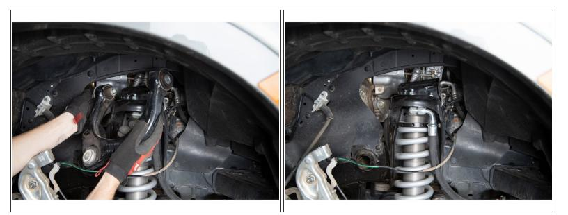
• Remove the upper control arm assembly from the vehicle.
