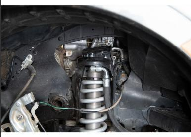
Remove the upper control arm assembly from the vehicle.
