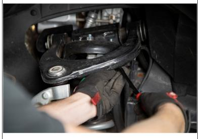
Carefully pull the ABS wire retainer from the upper control arm with a flat head screwdriver.
