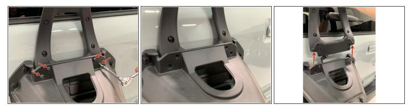
• Remove the four screws securing the 3rd Brake Light Bracket using a T30 Torx bit.
