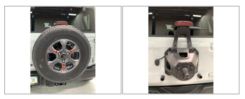
• Remove the spare tire from the vehicle to expose the 3rd brake light mounting bracket.
