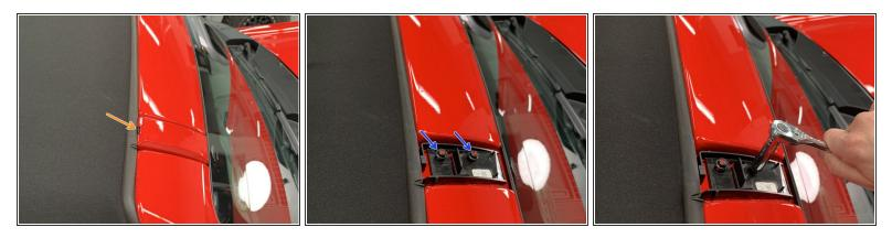
• Remove both Windshield Accessory Mount Caps by pushing inward on plastic tab.
