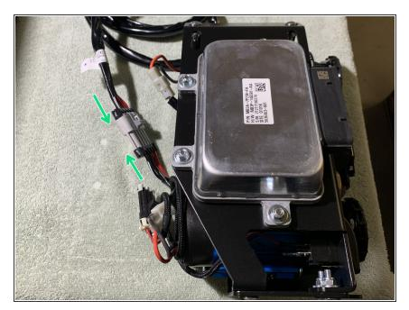
Connect the ARB Power Harness to the ARB Twin Compressor.
