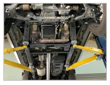
If there are any factory skid plates on the vehicle that would prevent installation of this skid plate, remove them.
