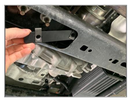
Install the two clip nut tabs into the crossmember just in front of the transfer case and align with the round holes.
