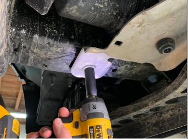
\*If equipped\* Using a 15mm wrench/socket, remove the two bolts securing the silver lower intercooler mount to the underside of the frame.
