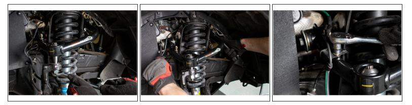
• Pivot the tapered stem so that it lines up with the tapered hole in the spindle. Push the upper control arm downward so the tapered pin engages the spindle.
