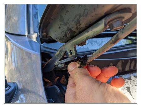
On the right side hood hinge there is a washer line clip that needs to be removed to access the bolt head.
