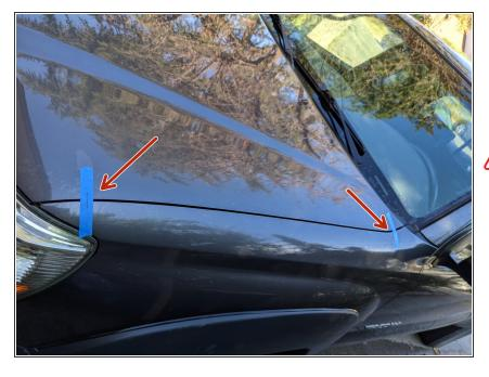
The Light Mounts require the hood hinge bolts to be loosened. The hood hinge is slotted to allow hood alignment. If the hood is improperly aligned, the hood will not open properly and may become stuck closed. Be careful to make sure the hood stays in position during the install.
