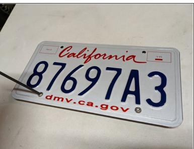
Install your license plate on the plate bracket. The cage nuts go on the bottom, as shown in the photos. Snug hardware but do not fully tighten yet.
