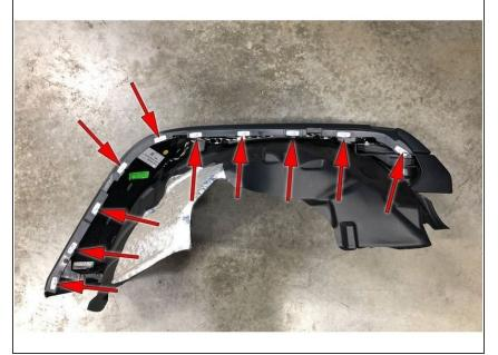
• There are ten retaining clips on the backside of the flare. These clips may be damaged during disassembly. Replacement clips are available from Jeep dealers, part number 68526185AA.
