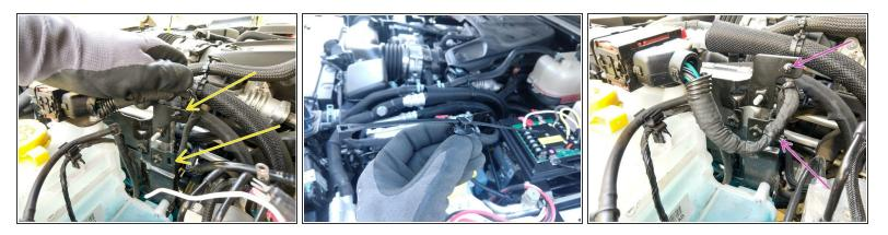
(i) The 3.6 V6 engine needs to have a wiring harness moved before installing the controls plate.
