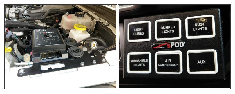
• After the sPOD install has been completed, turn on the compressor using the sPOD control panel.
