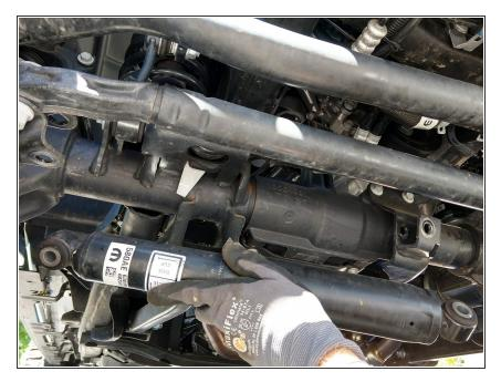
Remove the existing steering damper in order to verify the mounting width.
