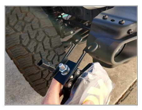
We recommend installing the chosen lights on the brackets before installing the brackets on the vehicle. Snug up light mounting hardware but do not torque at this time.
