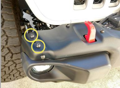
After identifying the left and right brackets, use a T45 torx driver to remove the 2 factory bolts on the top of the bumper, as shown. The bumper shown has had the outer 'wings' removed. Installation is the same if the wings are still in place.
