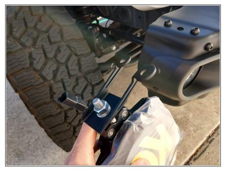
• We recommend installing the chosen lights on the brackets before installing the brackets on the vehicle. Snug up light mounting hardware but do not torque at this time.
