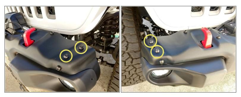
After identifying the left and right brackets, use a T45 torx driver to remove the 2 factory bolts on the top of the bumper, as shown. The bumper shown has had the outer 'wings' removed. Installation is the same if the wings are still in place.
