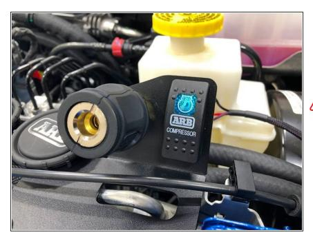
• Toggle the compressor switch to the on position. The compressor should turn on for a short period of time then turn off.
