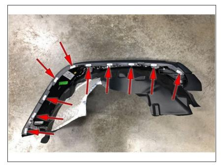
There are ten retaining clips on the backside of the flare. These clips may be damaged during disassembly. Replacement clips are available from Jeep dealers, part number 68526185AA.
