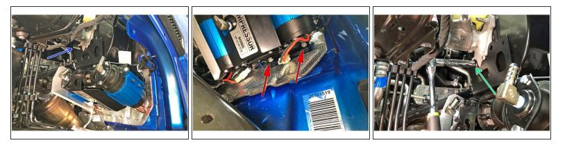
Install the compressor assembly onto the lower MC stud and the two firewall studs with the previously installed Grimm OffRoad spacer.
